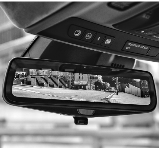
NEW TECHNOLOGY The rearview mirror in a Cadillac CT6 shows images from a camera mounted atop the car. The virtual cockpit in an Audi Q7 sport utility vehicle displays multiple functions on an LCD screen.
